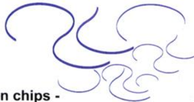
Loosely curled chips - Correct feed speed
